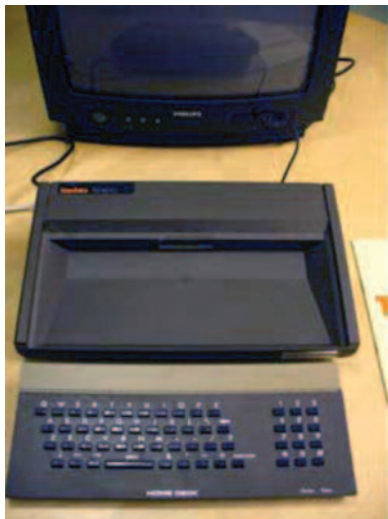
Tandata Td1400 Prestel terminal ( supplied by the Nottingham Building Society for its home banking service ).
